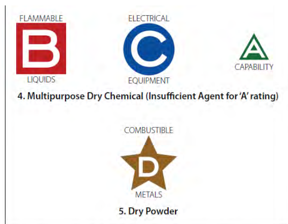
Figure 11-7. Typical extinguisher markings.
