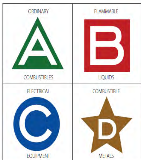
Figure 11-8. Identification of fire extinguisher type location.
