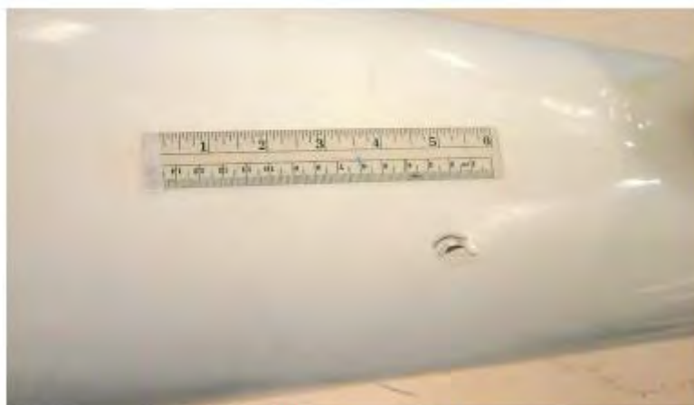
Figure 2-32. Digital image of impact damage.
