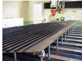
COBONDED ASSY OUT OF AUTOCLAVE, BEFORE STRINGER TOOLING DEMOULDING
