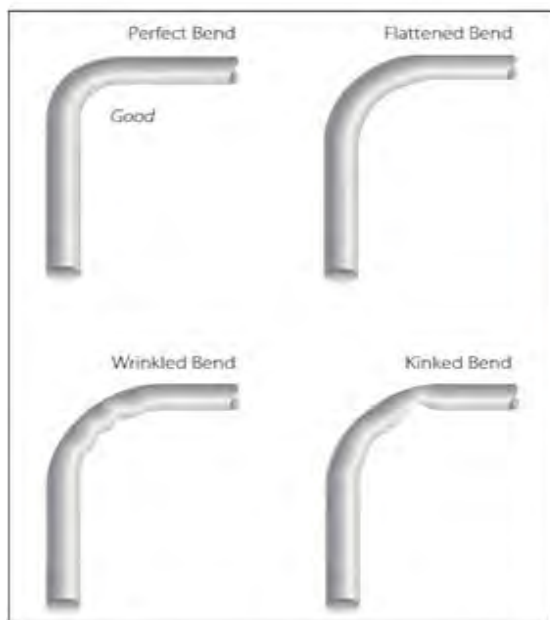
Figure 7-5. Correct and incorrect tubing bends.
