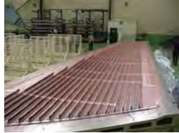
COBONDED ASSY OUT OF AUTOCLAVE, BEFORE STRINGER TOOLING DEMOULDING
